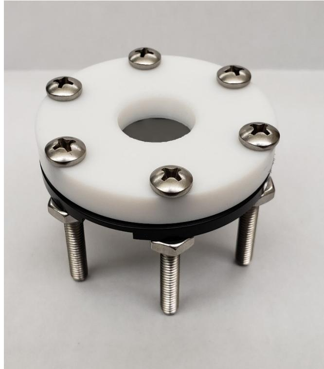
NOTE: Once the assembly is complete, leak check the Fixture by filling the well formed by the Teflon deposition mask and the surface of the FAC with water. Allow this to sit for at least 30 minutes and ensure there are no leaks prior to proceeding with corrosive solutions. This is especially important when using the Electroless Deposition Fixture for the first time.
