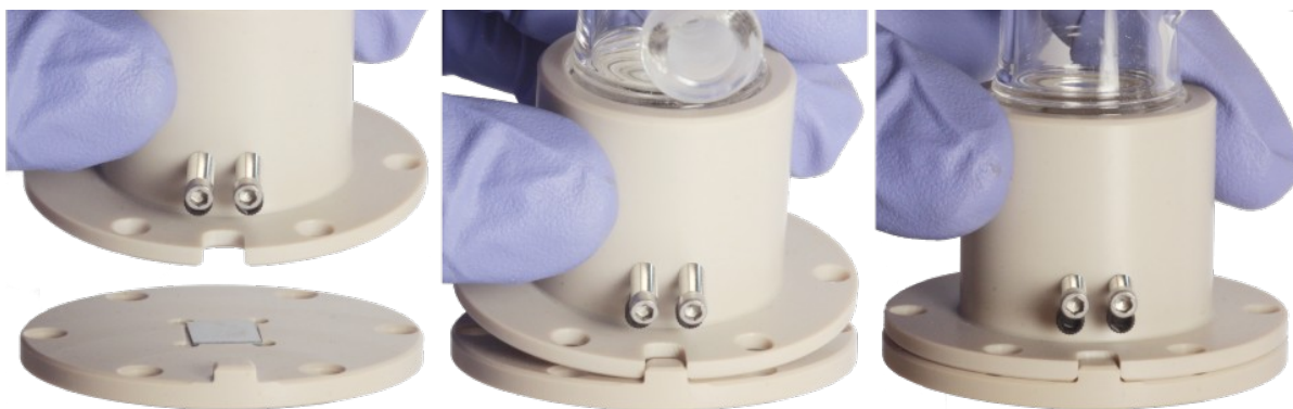
Fig. 9) Sealing the wafer in the cell. This step should be done with the wafer holder installed in the VeeMAX III top plate (not shown for clarity).
