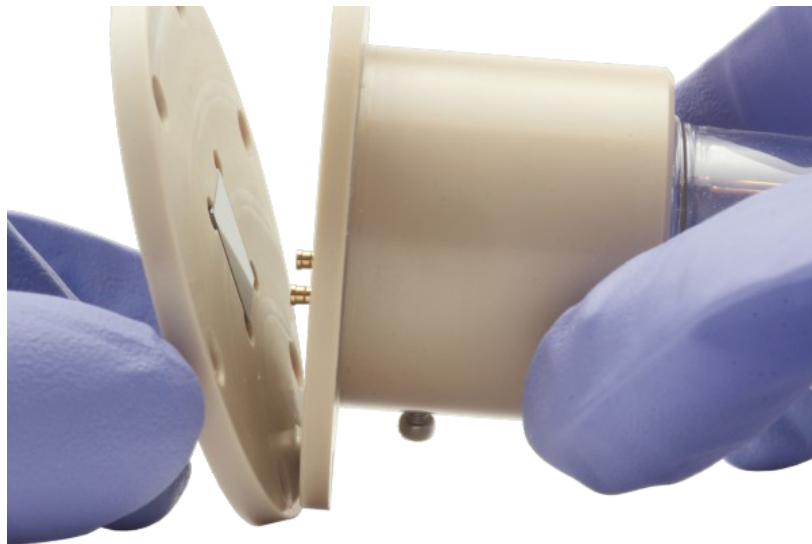
Fig. 11) Alternative, more challenging assembly method to mitigate the risk of breaking wafers without using the nylon pin-retaining screws.
