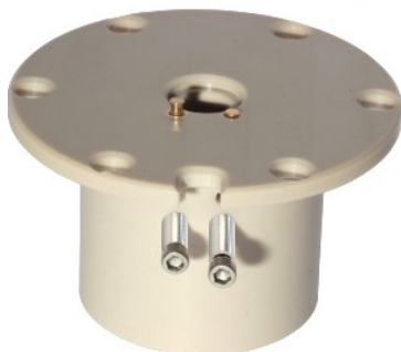
Fig. 7c) The left pin protrudes correctly, however the right pin has sunk to the bottom of the hole because the contact screw was inadequately tightened.
