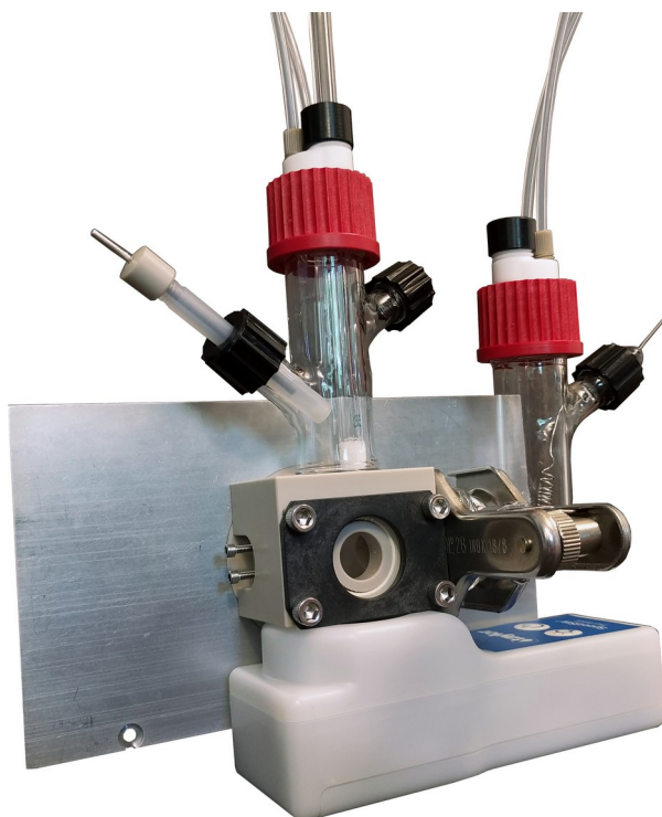
Assembled Jackfish J4 H-cell.
