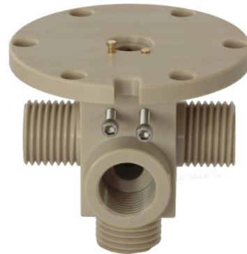
Figure 1b) The right pin protrudes correctly, however, the left pin has sunk to the bottom of the hole because the contact screw was tightened inadequately.
