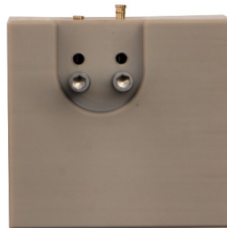
Fig. 2b) The right pin protrudes correctly, however the left pin has sunk to the bottom of the hole because the contact screw was inadequately tightened. Note: the counter electrode compartment assembled in the preceding step is omitted for clarity.
