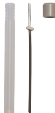
Figure 2: Unscrew the cap and remove the wire and O-ring to fill the reference electrode.
