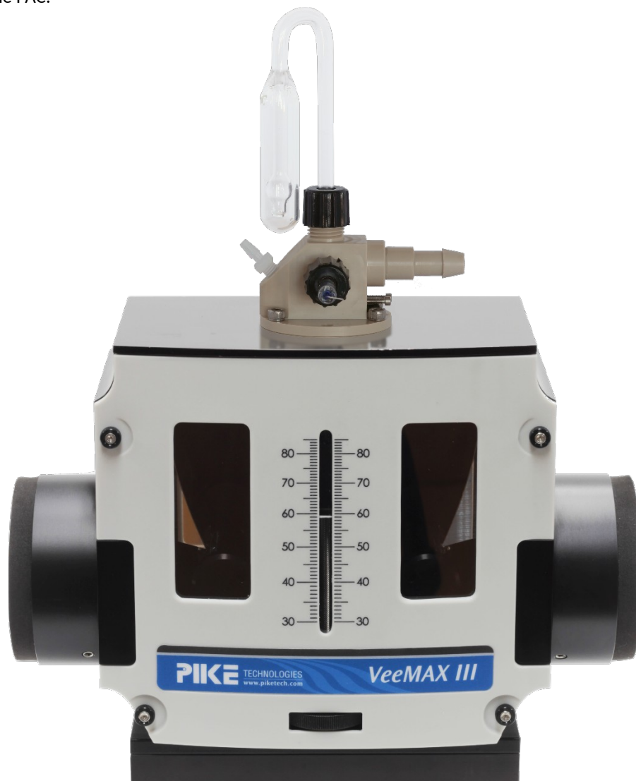
Jackfish Easy Electrochemical “Eel” Flow Cell assembled on the VeeMAX III accessory.
