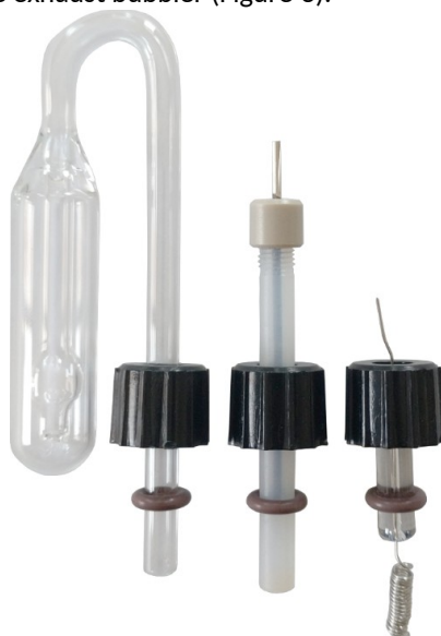
Figure 3) Caps and O-rings installed on accessories.
