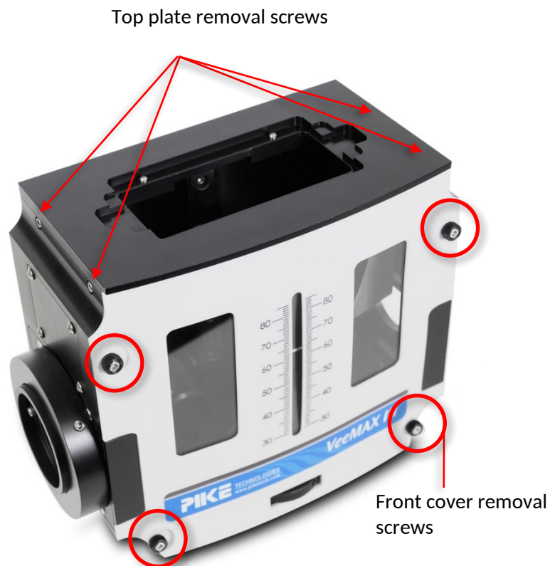
Figure 10) VeeMAX III shown with removable standard top plate.
