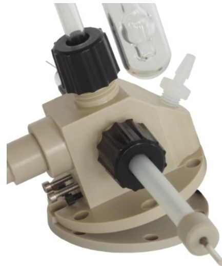
Figure 7) Sealing the wafer in the cell. This step should be done with the wafer holder installed in the VeeMAX III top plate (not shown for clarity).
