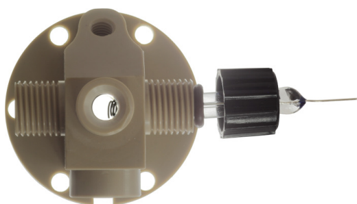
Figure 5(a): When installing the counter electrode, look through the top port and confirm that the wire is visible when the O-ring is seated on the accessory port (adjust position of the O-ring on the shaft if necessary). The reference electrode should be just barely visible through the top port and should not interfere with the counter electrode.
