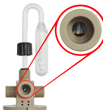
Figure 5(b): Look through the outlet port when installing the gas trap. In this case, the bubbler has been installed too deeply into the cell and it is blocking the outlet port.
