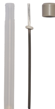
Figure 16: J2 reference electrode: unscrew the cap and remove the wire and O-ring to fill the reference electrode.
