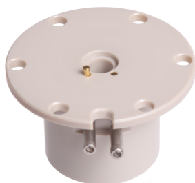
Figure 8(c): The left pin protrudes correctly, however the right pin has sunk to the bottom of the hole because the contact screw was inadequately tightened.
