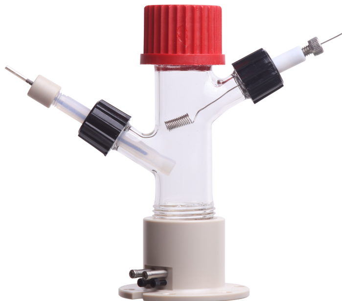
Figure 17: Complete J2WP cell assembly.
