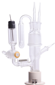
J1 Spectroelectrochemical Cell
