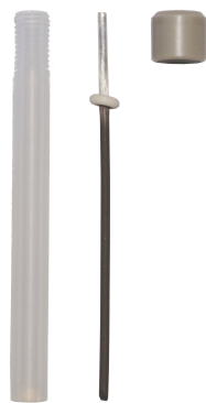
Figure 2: Unscrew the cap and remove the wire and O-ring to fill the reference electrode.
