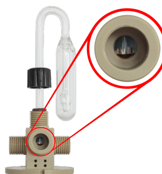
Figure 4(b): Look through the outlet port when installing the gas trap. In this case, the bubbler has been installed too deeply into the cell and it is blocking the outlet port.
