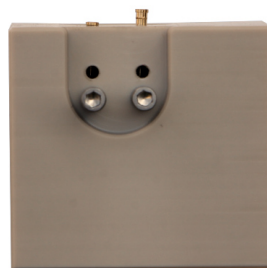
Figure 3(b): The right pin protrudes correctly, however the left pin has sunk to the bottom of the hole because the contact screw was inadequately tightened. Note: the counter electrode compartment assembled in the preceding step is omitted for clarity.
