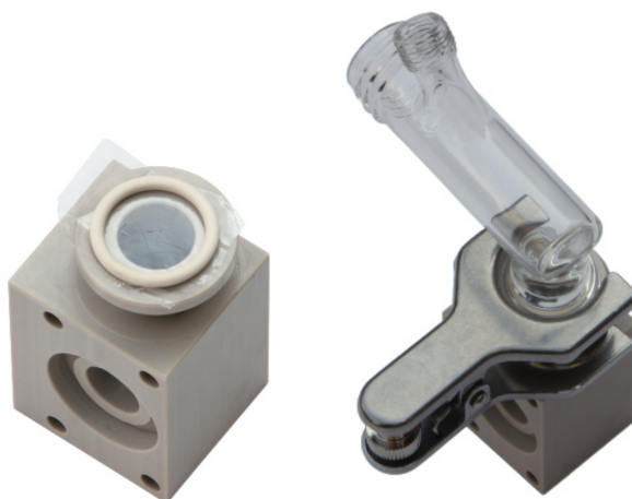
Figure 2: Attaching the counter electrode compartment.
