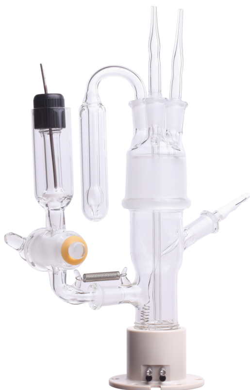
Figure 15: Complete J1FP cell assembly.
