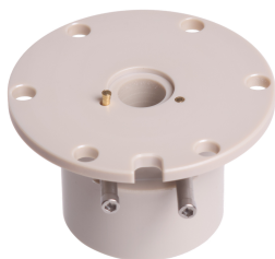
Figure 2(c): The left pin protrudes correctly, however, the right pin has sunk to the bottom of the hole because the contact screw was tightened inadequately.
