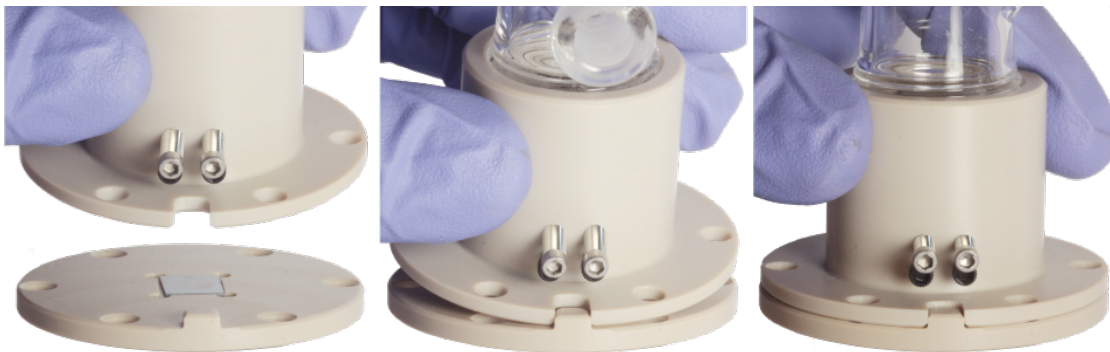
Figure 12: Sealing the wafer in the cell. This step should be done with the wafer holder installed in the VeeMAX III top plate (not shown for clarity).
