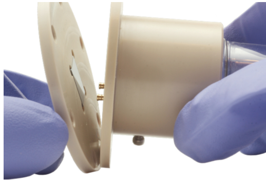
Figure 14: Alternative, more challenging assembly method to mitigate the risk of breaking wafers without using the nylon pin-retaining screws.
