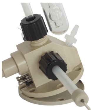
Figure 8: Sealing the wafer in the cell. This step should be done with the wafer holder installed in the VeeMAX III top plate (not shown for clarity).
