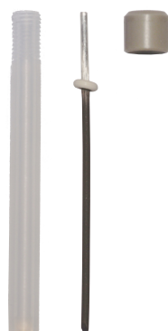
Figure 7: Unscrew the cap and remove the wire and O-ring to fill the reference electrode.
