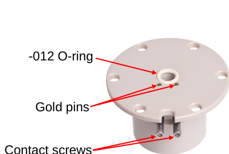
Figure 8(a): Install the -012 O-ring in the pocket on the underside of the cell base.
