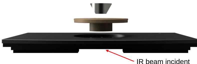
Figure 4(b): Orientation of FAC in crystal holder in top plate.
