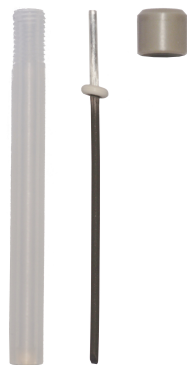
Figure 8: Unscrew the cap and remove the wire and O-ring to fill the reference electrode.
