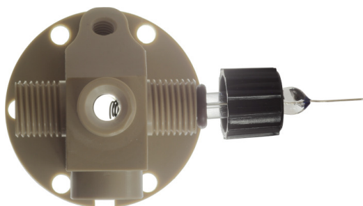
Figure 4(a): When installing the counter electrode, look through the top port and confirm that the wire is visible when the O-ring is seated on the accessory port (adjust position of the O-ring on the shaft if necessary). The reference electrode should be just barely visible through the top port and should not interfere with the counter electrode.
