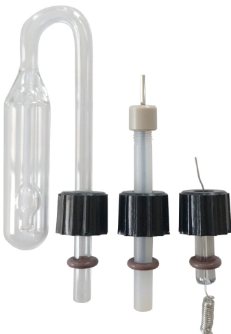
Figure 3: Caps and O-rings installed on accessories.
