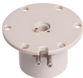
Figure 7(c): The left pin protrudes correctly, however the right pin has sunk to the bottom of the hole because the contact screw was inadequately tightened.
