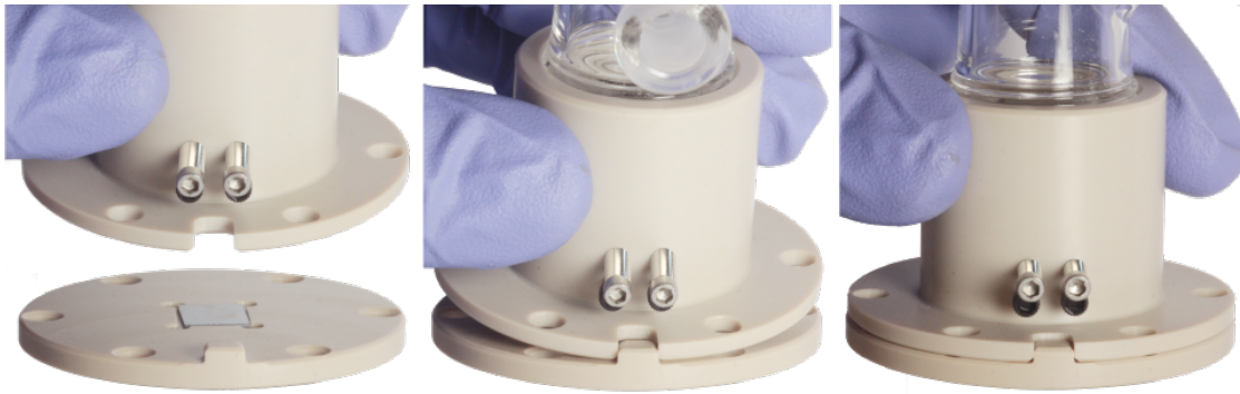
Figure 10: Sealing the wafer in the cell. This step should be done with the wafer holder installed in the VeeMAX III top plate (not shown for clarity).
