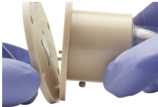
Figure 12: Alternative, more challenging assembly method to mitigate the risk of breaking wafers without using the nylon pin-retaining screws.
