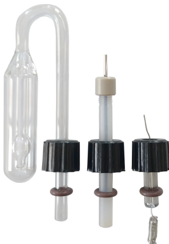
Figure 3: Caps and O-rings installed on accessories.
